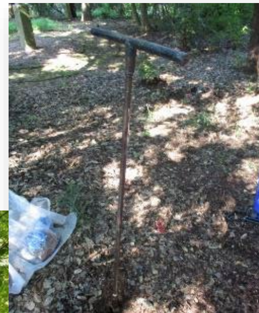
Above – Discrete subsurface soil sampling by hand auger. Soil Remedial Action. Spring Valley FUDS, Washington, D.C.
